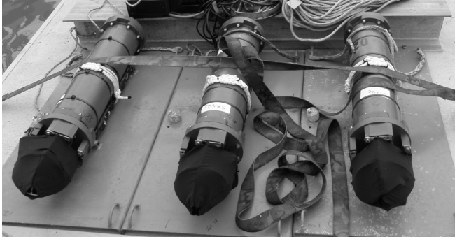
FIG. 2. AMAR recorders on steel base plates ready for deployment in the Tappan Zee River. Spandex flow shields cover the hydrophones to help reduce pseudo-noise from river currents moving water around the hydrophones.
